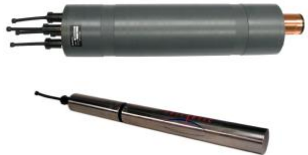
Fig. 1. ISUS nitrate sensor PVC version with copper bio-fouling guard (top) and stainless steel SUNA (below).
