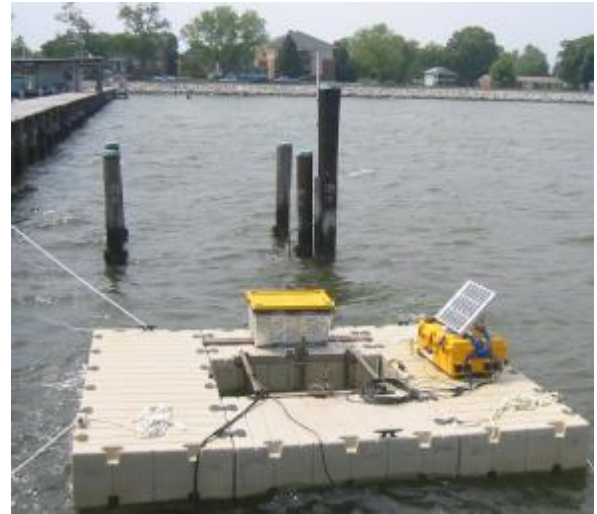
Fig. 5. ACT instrument mooring at the Chesapeake Bay Laboratory pier.
