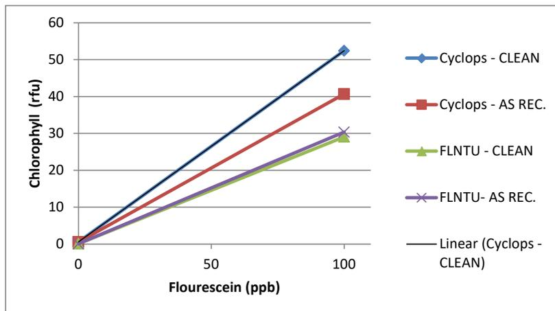
There was no appreciable fouling on FLNTU over the course of the deployment. While the readings did reveal fouling on the Cyclops sensor, it was left in place on the buoy for a couple of months after the available data ends. The data do not reveal any apparent patterns of fouling (shifts in baseline, etc.) and it is likely that the fouling revealed in the 'as recovered' measurements occurred after the existing data were collected.
