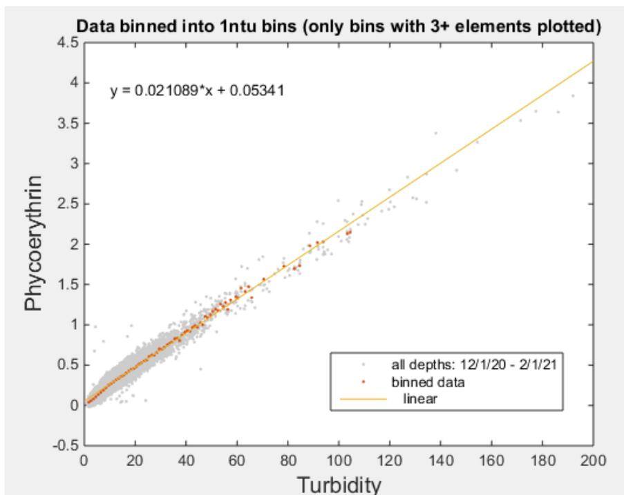
$$\text{Corrected PE} = \text{raw PE} - (\text{turbidity} * 0.0211 + 0.0534)$$
